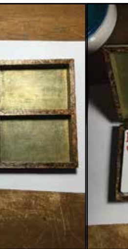
Box top showing completed steps of lining, scribing and edging.
